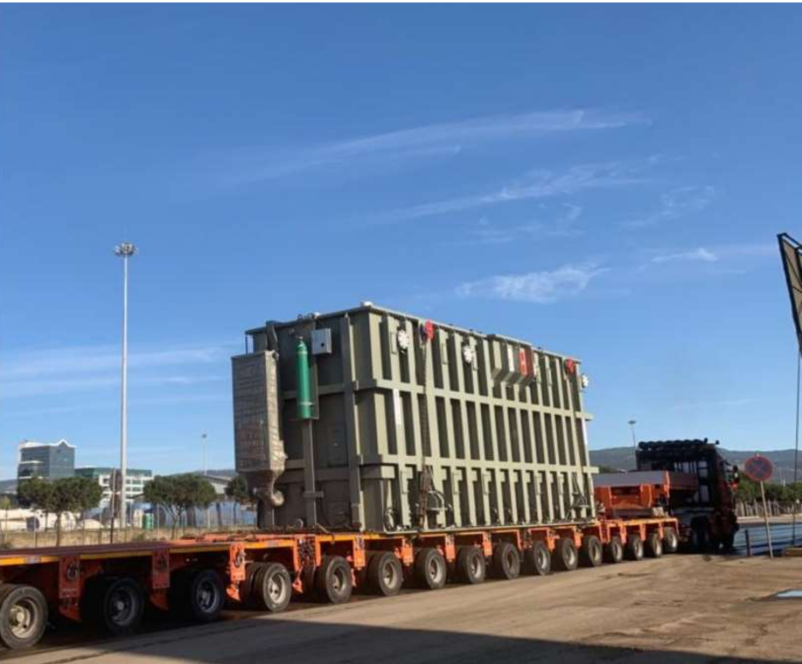
E #24 Power Transformer 280 MVA/400 1 x unit 10095x4120x4315mm / 240T Thessaloniki port Scope: FOB till FOT & transit customs formalities to NMK
